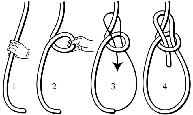
After the bowline has been formed, you must tighten it correctly like this.
